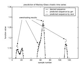
Figure 4. A higher room-in plot has clearly shown the overshooting results from GM(1,1) prediction marked by •. In contrast, ASVR has perform very well in the prediction of G-M chaotic time series without any overshooting problem and its predicted results are indicated by  $\times$ .
