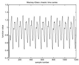
Figure 1. The Mackey-Glass chaotic time series for 1201 sample points as a benchmark of complex time series prediction.
