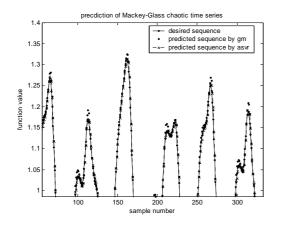
Figure 3. A room-in plot shows that the overshooting phenomenon has occurrence indicated by  $\bullet$  from GM(1,1) predicted results around the turning-point region.
