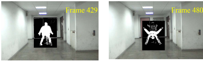
Fig. 6. Object extraction result of right-hand-side person in the Hall sequence using the proposed method.
