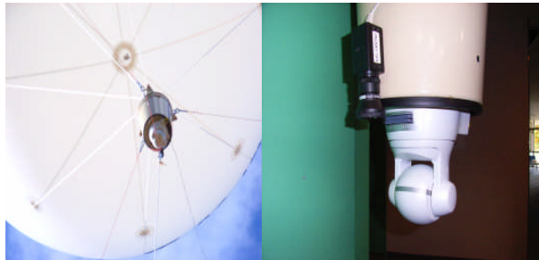
Fig. 5. Ballooned Omni-directional Camera System
