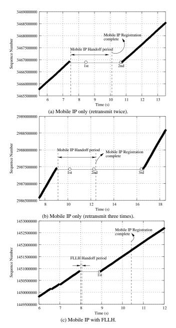
Fig. 7. TCP Packet Transmission Experiment.
