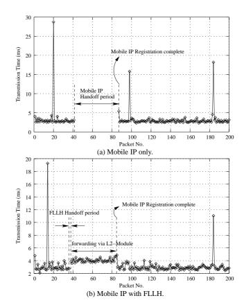
Fig. 6. UDP Packet Transmission Experiment.
