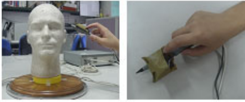
Figure 12: The 3D styling tool needs two sensors: one sensor is attached to a plastic head model, and the other one is used for controlling the editing tool.
