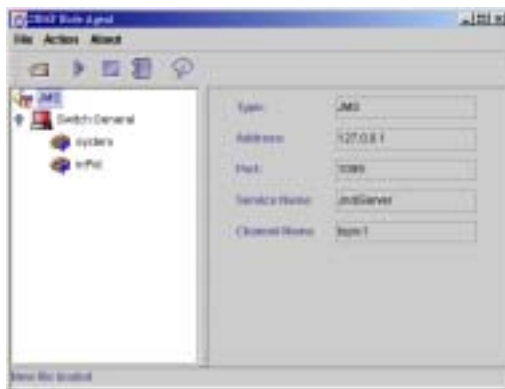
Figure 8: MDE Server. The left part shows the events received. The right part shows the configuration of the server.
