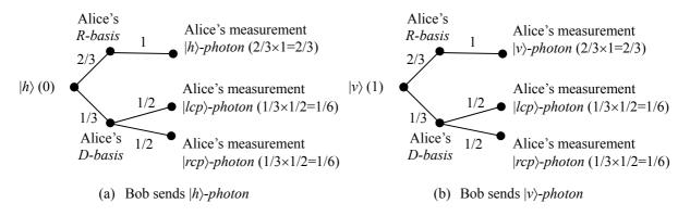
Figure 3. Analysis of idealized maximum efficiency for FEQKD protocol with Bob using *R-basis*.
