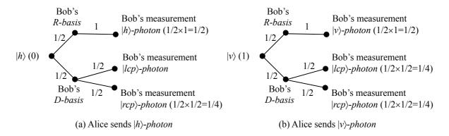
Figure 2. Analysis of idealized maximum efficiency for BB84 protocol with Alice using *R-basis*.
