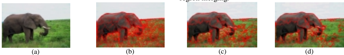
Fig.10 The results of Elephant in size 384x256 (a) The original image. (b) Automatic seeds generation and SRG. (c) Texture elimination by local edge and region merging. (d) Texture elimination by global edge and region merging.
