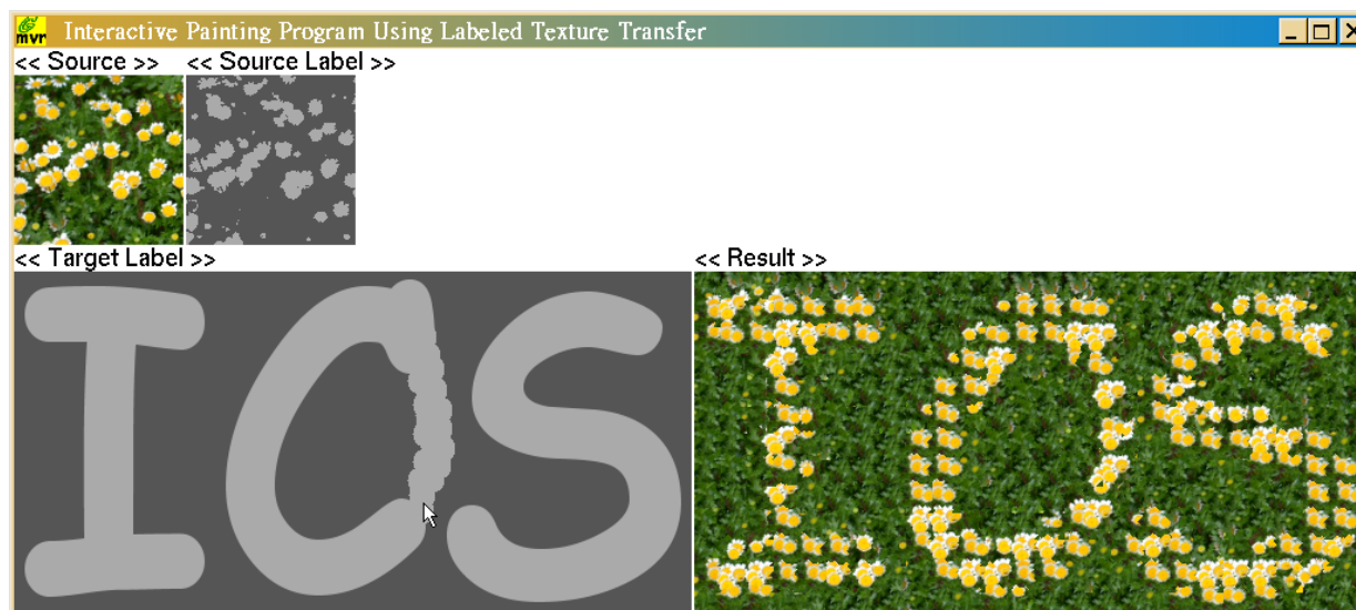
Figure 10: We develop an interactive system for the interested user painting the target label map to control the synthesis. Benefiting from one patch sampling at a time, we can provide the immediate update by issuing a query to the established kd-tree.
