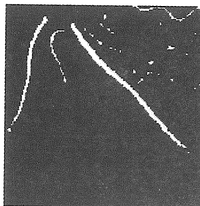
Fig. 4 After a bell-shaped filter and automated thresholding apply on Fig. 3.
