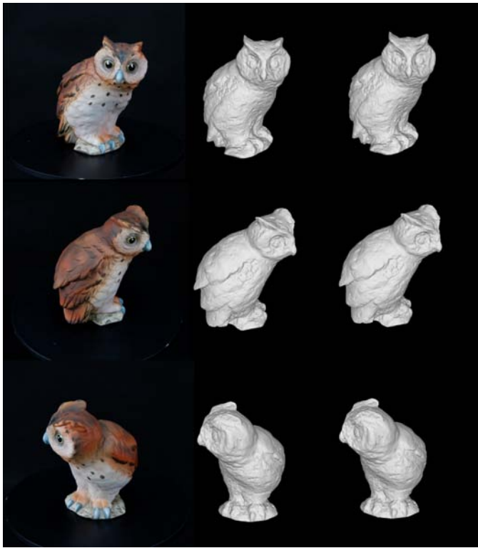
Fig. 9. Toy owl. Left column: image sequence. Middle column: similar viewpoints of the model reconstructed via volumetric graph cut with photo-consistency constraints alone. Right column: similar viewpoints of the model reconstructed via volumetric graph cut with both photo-consistency and silhouette constraints.
