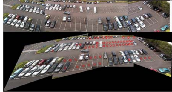
Fig. 21 The result of parking space detection by using color-four regions method
