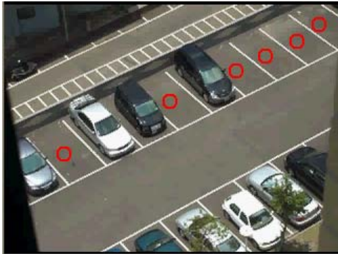
Fig. 24 The result of parking space detection in different scene
