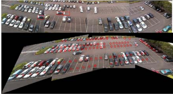
Fig. 19 The result of parking space detection by using edge-four regions method
