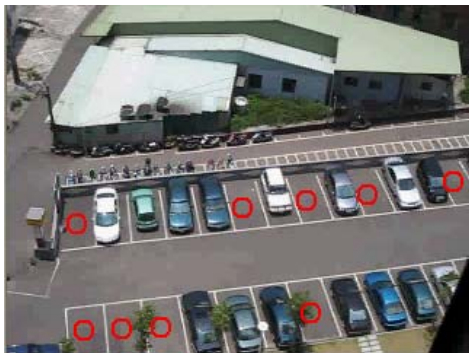
Fig. 25 The result of parking space detection in different scene
