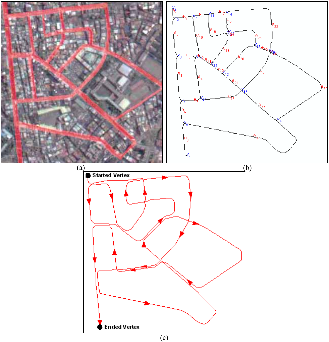
Fig.3. Route Planning for Waste Collection: (a) Red lines represent the selected streets where the vehicle drives; (b) initial graph; and (c) the final route is found by using the proposed method.
