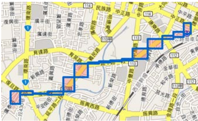
Figure 3. A trajectory represented by a series of boxes
