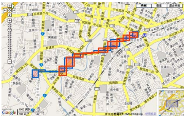
Figure 10. RAD algorithm monitoring incoming data-points against norms (in blue boxes) using box modeling
