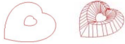
Figure 10 The cyclographic map for a closed domain with loop (a) boundary curve with MAT (b) Cyclographic Map
