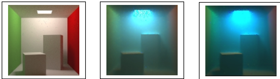
(a). Without participating media (b). Rendering participating media with 5 samples of wavelength. (c). Rendering participating media with 80 samples of wavelength. The color of participating media is more blueish than the color of participating media in Fig. 4(b).
