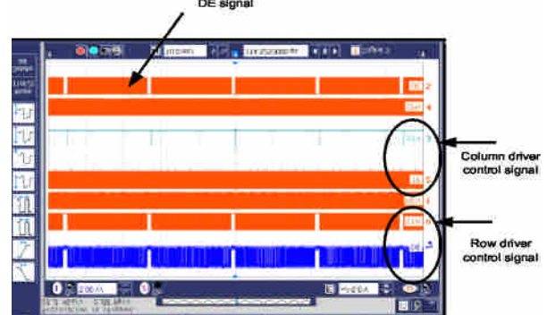
Figure18. Row and column driver control signal for FPGA verification.
