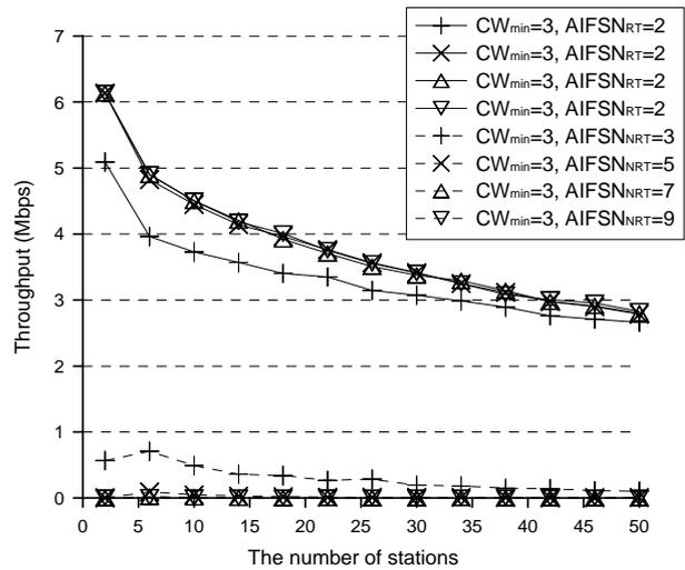
Fig. 4 Throughput versus the number of stations ( $CW_{min}=3$ )
