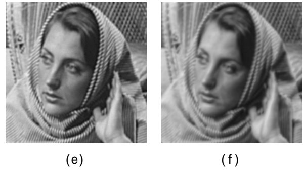
Fig.9.(a)Original Barbara image(zoom in), (b)Blurred Barbara image, (c)proposed method( s=5, c=0.4 ), (d)FSD method( s=3, c=0.45 ), (e)FSD method( s=5, c=0.4 ), (f)Gaussian method( 0.04 \times G_{0max} ).
