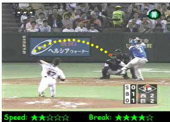
(a) Pitch frame of the first ball of the extracted trajectory with tracked ball positions superimposed on the frame
