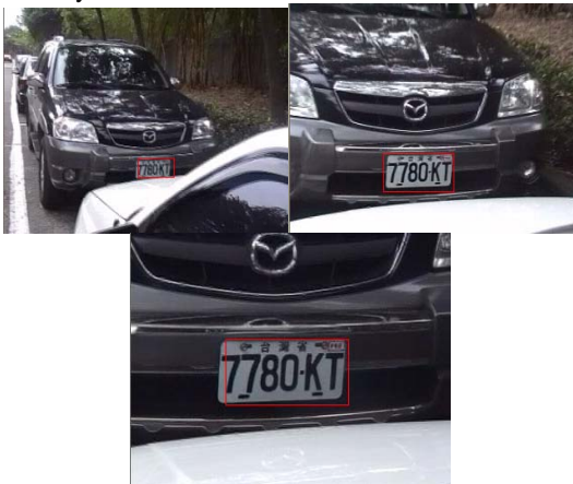
Fig. 10: Result of license plate detection when a video sequence was handled.
