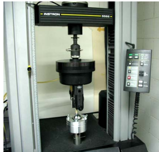
Fig. 1. A photograph of the fabric bagging tester
