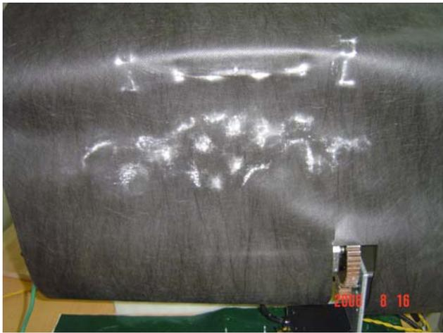
Fig. 2. Electrospun jet mutually repulsive deposition on supporting material
