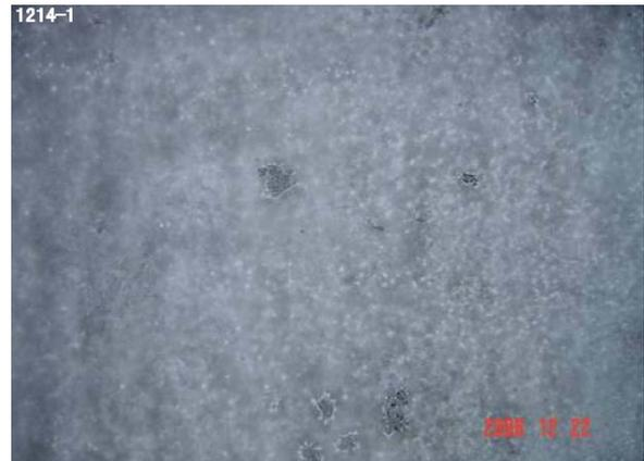
Fig. 8 The electrospun fiber could not fully deposit to fill up the aperture at low BW of nanofiber-film.
