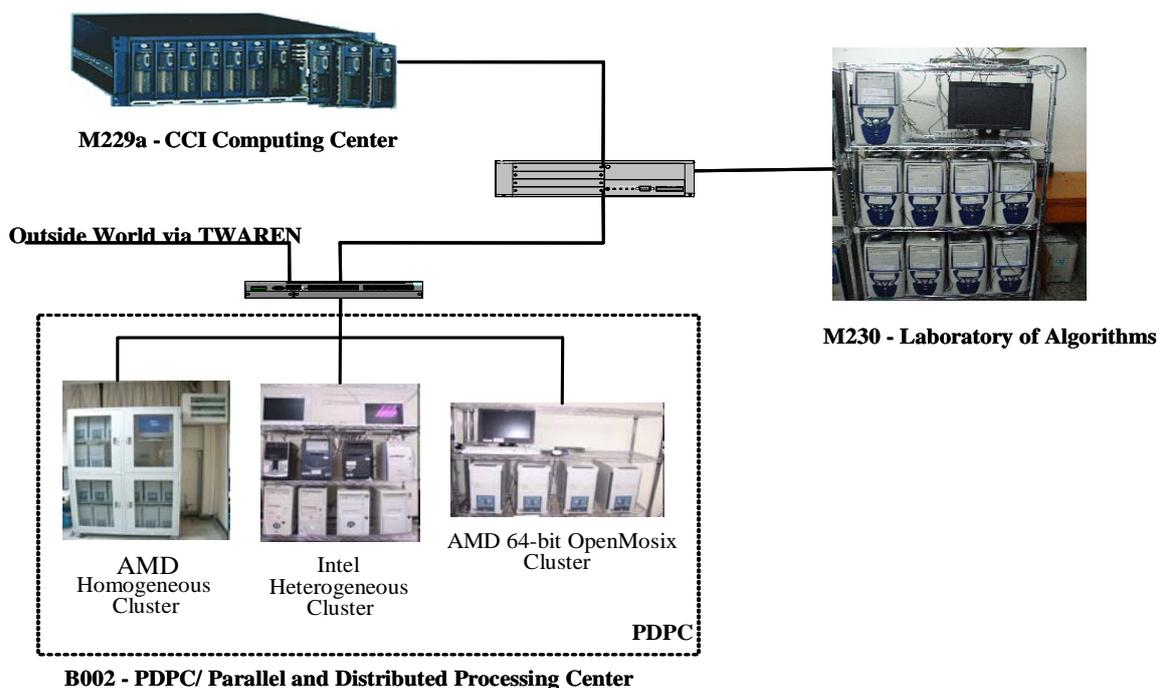
Fig. 1. The PCGrid grid computing infrastructure
