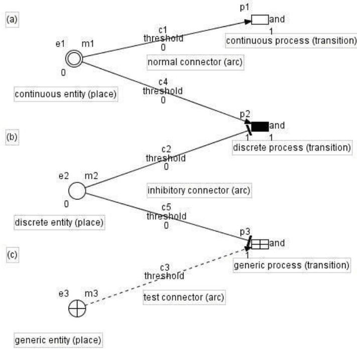
**Fig 1.** The different kinds of entities, processes, and connectors in HFPN. (a) continuous entity, normal connector, and continuous process. (b) discrete entity, inhibitory connector, and discrete process. (c) generic entity, test connector, generic process.
