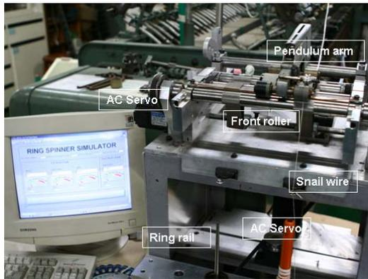
Fig. 1 Experimental ring spinning system
