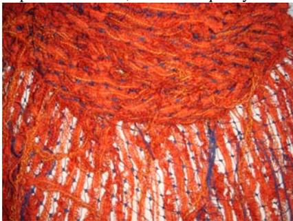
Fig 2. Fabric constructed using interweaving technique
