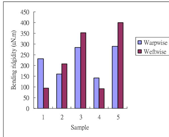
Fig. 4. Bending rigidity of spacer samples
