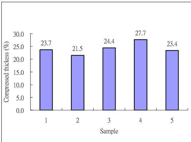
Fig. 3. Compressed thickness of spacer samples
