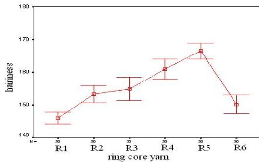
Fig4- effect of filament pre-tension on hairiness of ring core yarns
