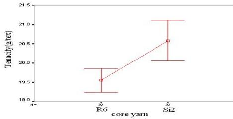
Fig 14- Comparison of tenacity of ring & siro core spun yarns
