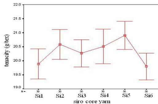
Fig 9- effect of feed position of core filament on tenacity of siro core yarn
