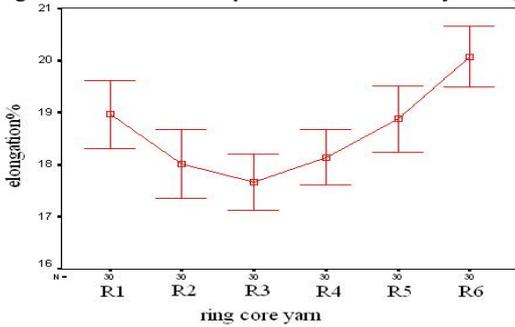
Fig 3- effect of filament pre-tension on percent of elongation of ring core yarns
