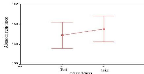
Fig 17- Comparison of abrasion resistance of ring & siro core spun yarns
