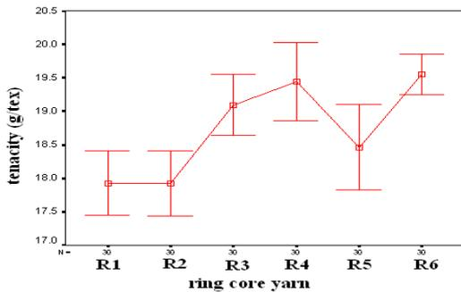
Fig 2- effect of filament pre-tension on tenacity of ring core yarns
