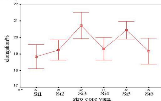
Fig 10- effect of feed position of core filament on percent of elongation of siro core yarn
