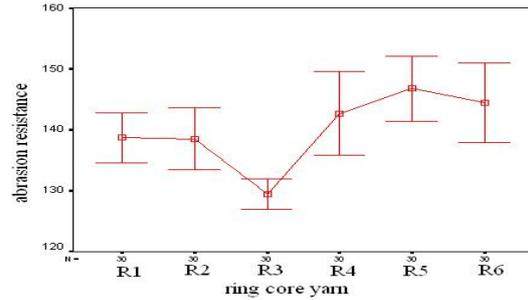
Fig5- effect of filament pre-tension on abrasion resistance of ring core yarns
