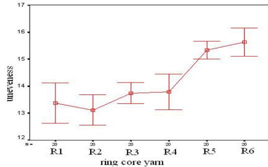
Fig6- effect of filament pre-tension on unevenness of ring core yarns
