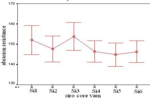
Fig 13- effect of feed position of core filament on abrasion resistance of siro core yarn
