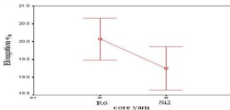
Fig 15- Comparison of elongation of ring & siro core spun yarns
