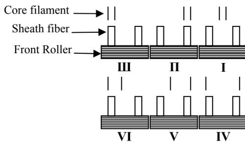
Fig1- different states of feed of core filament on siro core yarns
