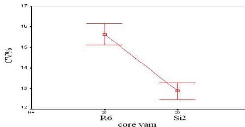
Fig 18- Comparison of unevenness percent of ring & siro core spun yarns
