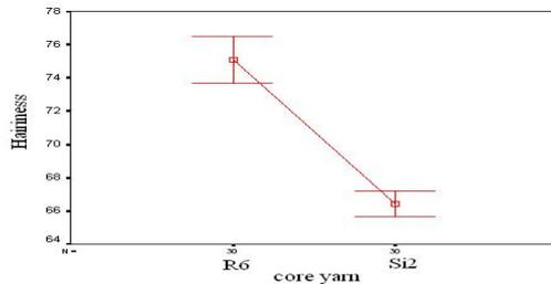
Fig 16- Comparison of hairiness of ring, & siro core spun yarns
